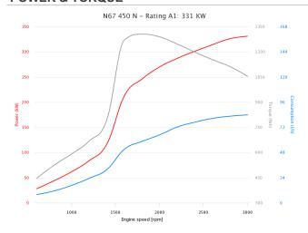
\* Net Power at flywheel according to ISO 8665, after 50 hours running, Fuel Diesel EN 590. Power tolerance 5%.
